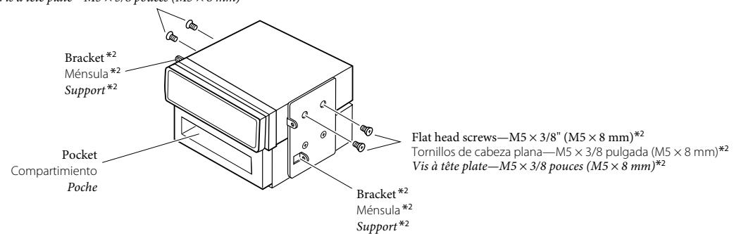
**Note** : When installing the unit on the mounting bracket, make sure to use the 3/8" (8 mm) -long screws. If longer screws are used, they could damage the unit.
